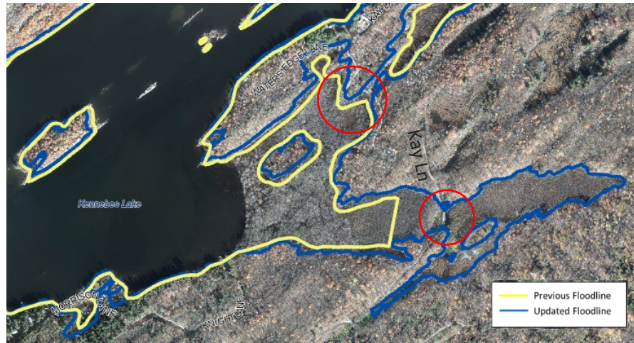
FIGURE 4-6: KENNEBEC LAKE SOUTH SHORE ALONG KAY LN
