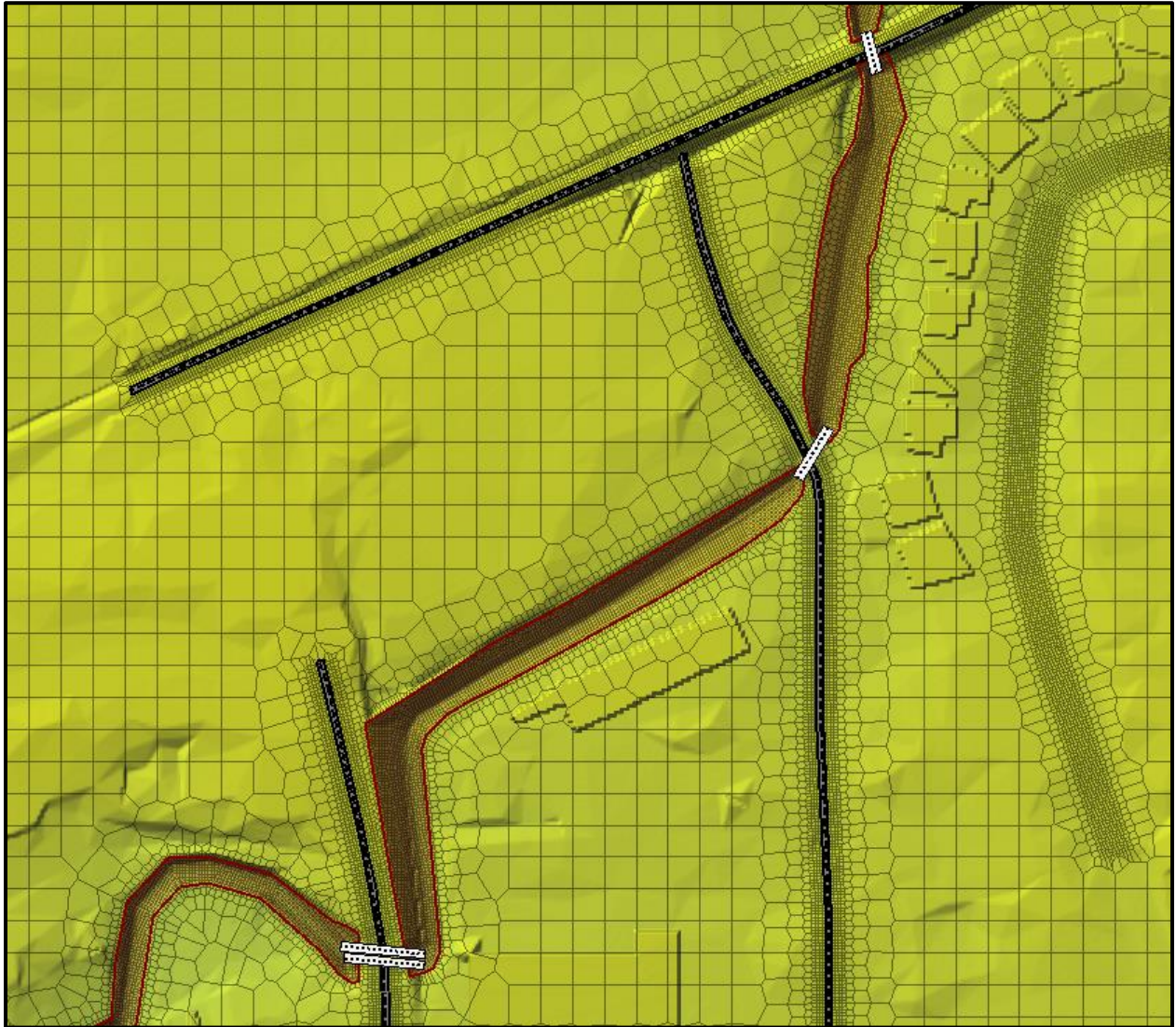
Figure 3-1: Example of Computational Mesh near Lake Breeze Ct. and Maple Ave with Refinement Regions for Channel and Overbank Areas
