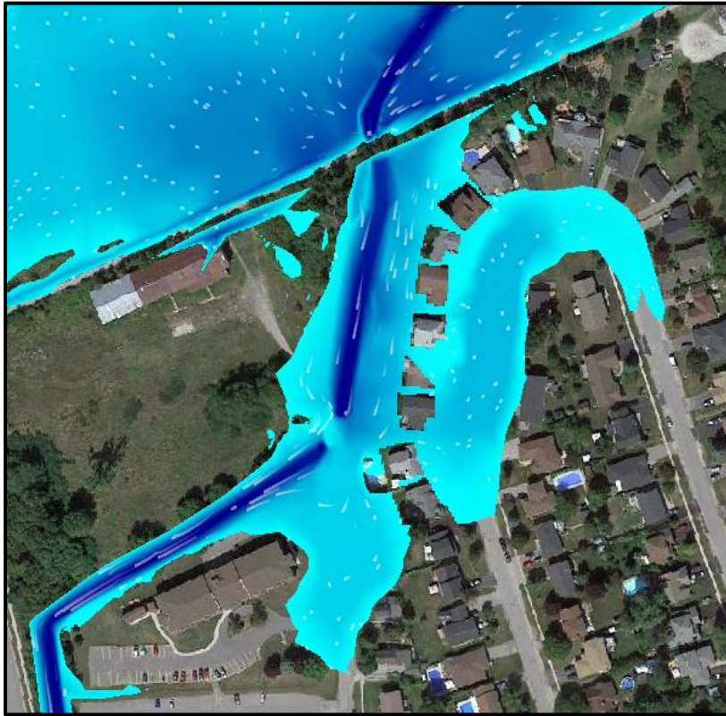
Figure 3-11: Schematic of Inundation Area Upstream of Maple Avenue
