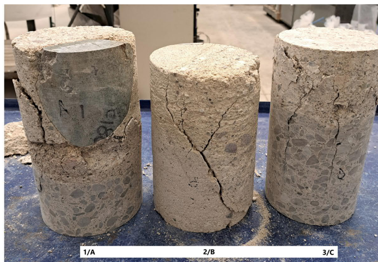
Figure 3-6: Cores after Compressive Testing
