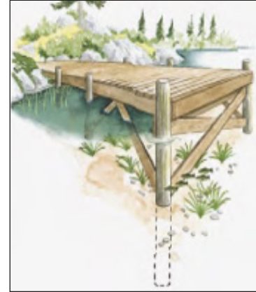
Figure 8: Permanent Post Dock
