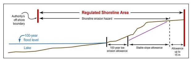
Figure 13: Lake Erosion Hazard
