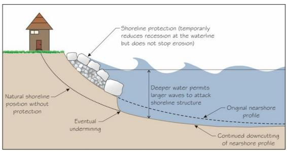
Figure 14: Lake Erosion Down Cutting
