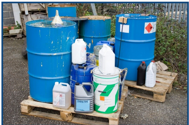
These chemicals are not properly stored. Chemicals and liquid waste should be stored safely using a drip catching tray.
