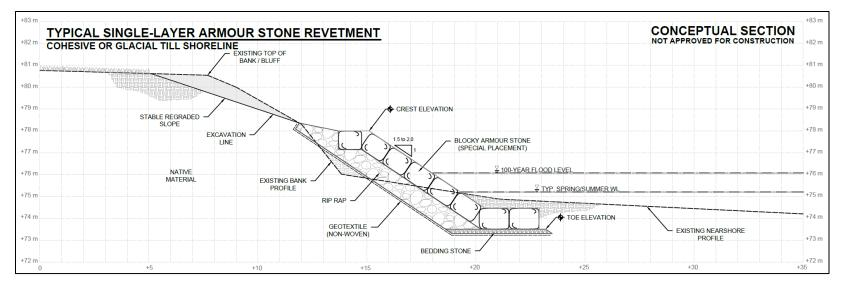
Figure 7.17 Typical single-layer armour stone revetment for a cohesive or glacial till shoreline (concept only)
