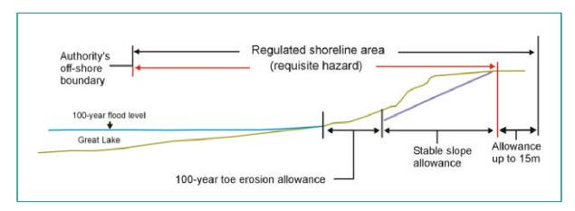
Figure 5.1 Erosion hazard setback approach
