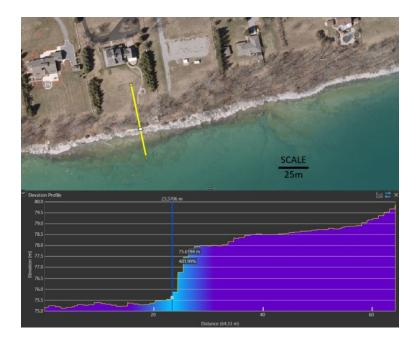
• Map 100-years of Future Recession: The 100-year recession rate was mapped by buffering the toe of slope line by a distance equal to 100 times the average annual recession rate outlined in Section 4.2.2.
