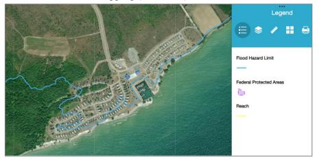
• Erosion of the bedrock banks threatens residential developments on Salmon Point Road where buildings are located too close to the top of bank. Shore protection must be well engineered to remain stable on the bedrock shoreline and withstand potential damage during severe storms.
