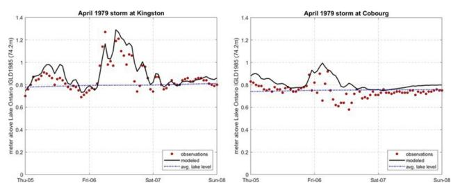
Figure 4.14 Measured (red dots) versus modelled (continuous black line) water levels at Kingston (left) and Cobourg (right) during the April, 1979 storm surge event (in metres above Chart Datum)
