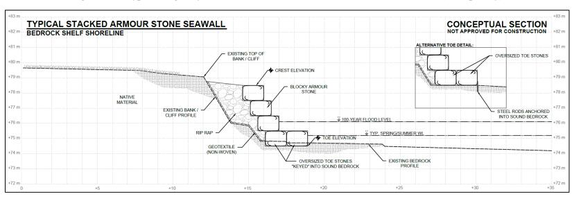
Figure 7.20 Typical stacked armour stone seawall founded on a bedrock shelf (concept only)
