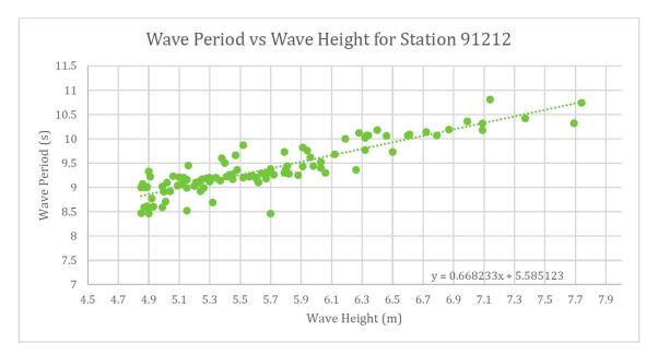
Figure 4.23 Relationship between significant wave height (Hs) and wave period (Tp) for top 100 storm events at WIS Station 91212
