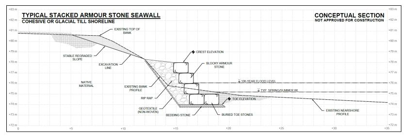
Figure 7.21 Typical stacked armour stone seawall for a cohesive or glacial till shoreline (concept only)
