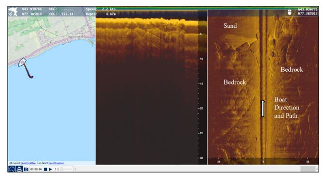
Figure 3.17 Sonar imaging of lake bottom near Wellington
