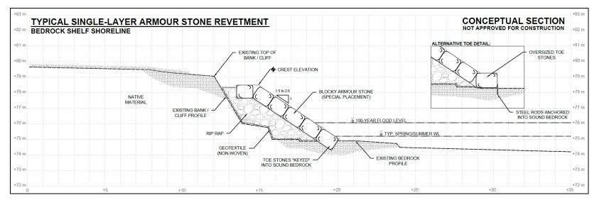
Figure 7.19 Typical single-layer armour stone revetment founded on a bedrock shelf (concept only)
