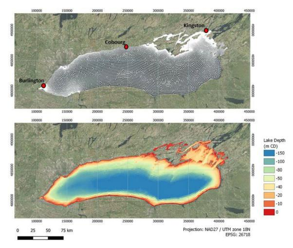
Figure 4.11 Lake Ontario surge model mesh (top) and interpolated bathymetry (bottom)
