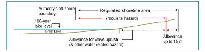
Figure 5.2 Flooding hazard definition
