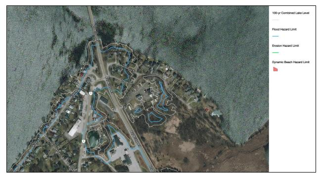
Figure 5.3 Sample of flood hazard mapping for a low-lying area at the southern end of the Belleville Bridge (white line is the 100-year flood level and blue line is the flooding hazard including wave uprush)
