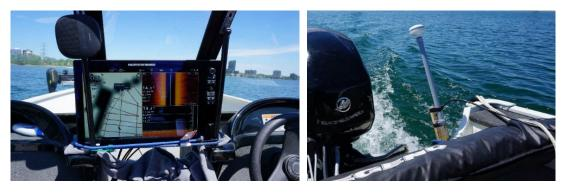
Figure 3.15 SOLIX data collection unit and transducer mount
