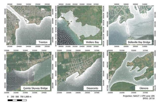
Figure 4.12 Mesh detail at specific locations of interest within the Bay of Quinte
