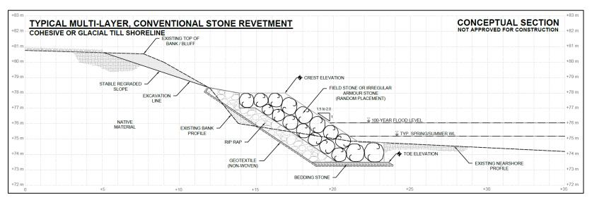
Figure 7.18 Typical multi-layer, randomly placed stone revetment for a cohesive or glacial till shoreline (concept only)
